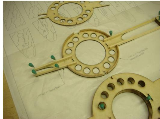
The rear spar is assembled in a similar fashion with 1/8"x 1/4" spruce spars. Leave the main spar pinned to the board.
