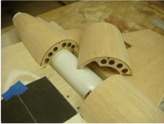
As the bottom is planked, cut between the main spar and N6A, and the rear spar and N6B to free the hatch. Glue N1 and N2 to the front of the nacelles and sand to shape. The inlet edge should have a smooth, round cross section to ensure good air flow into the fan.
