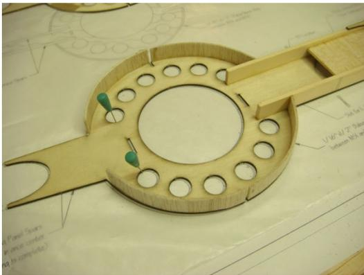
Cut several strips of 1/16"x1/2" balsa for shear webs between MS1 and MS2. Glue them in place and sand them flush with the spruce spars. Glue MS2A to MS2. Glue the MS2's and the other WJ1 in place.
