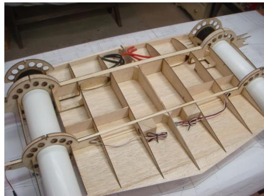
Route the aileron servo leads through the holes in R2 and through the rear spar. Sheet the top center section of the wing with 1/16" balsa. Carve and sand the L.E. to shape.
