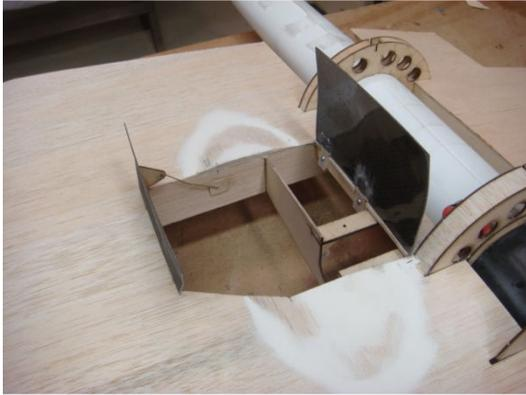
Cut the gear openings from the bottom sheeting. Cut the gear doors to shape and temporarily hinge them. The outer door will be secured to the gear strut and the inner door uses an over-center spring to hold it open and closed. The wheel hits a lever glued to the inside of the inner door to open and close it.
