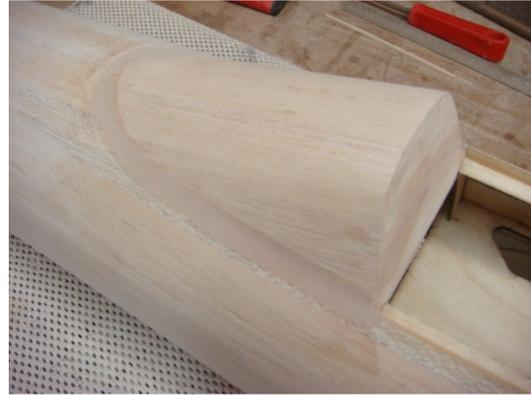
Rough trim the canopy to shape. Glue F6A in place and frame up the turtle deck. It is sheeted/planked with 1/16" balsa. Cut a floor for the cockpit and install the canopy as shown on the plans.
