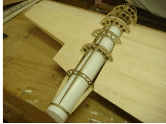
Cut two rear ducts and fit the remainder of the nacelle pieces in place (N6, N7, N8, and N9). Protect the N6 pieces from the spars and wing sheeting with wax paper.
