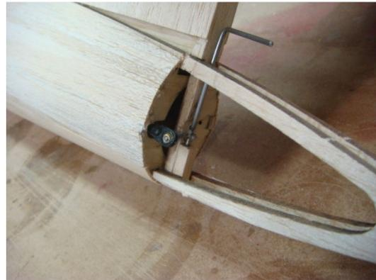
Install the rudder and elevator control rods.
