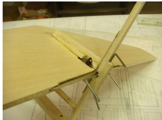
Glue the stab assembly in place on the fin assembly. Make sure it is square to the fin. Connect the elevator linkage and make any adjustments for smooth operation. Glue the V5/V6 assembly and
