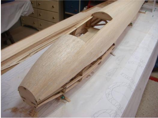
When the top and sides are done, the fuselage is removed from the board to finish up the bottom. Glue balsa block to the front of the fuselage and sand to shape.
