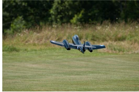
The stall is very gentle. With the throttle off and full up elevator, the stabilizer stalls before the wing and you get a series of “micro porpoise” motions until you relax the elevator or add power.
