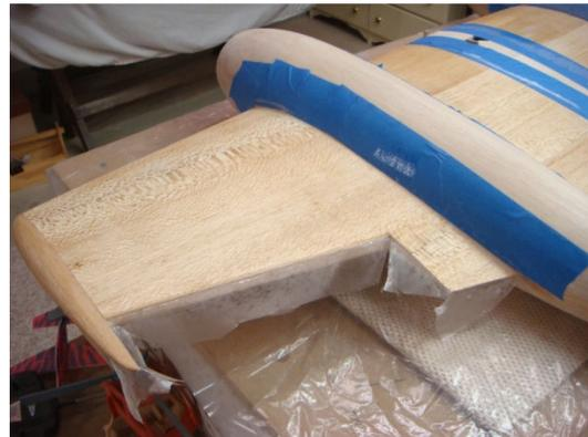
At this point the Meteor should be ready for finishing. The prototype was fiberglassed with 0.5 oz. cloth and painted. This is a short step on paper, but it took several weeks of sanding, filling, and priming to get ready for paint. I've come across several color schemes for a T.7 including scarlet red, Israeli camouflage, and the gloss black one that originally inspired me. This design could easily be bashed into one of the many other variants of the Gloster Meteor.
