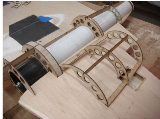
Plank the nacelles with 1/16" balsa. To help with this, a "gore" template is include on the plans. The shape of the gores will reduce the amount of trimming and fitting required.
