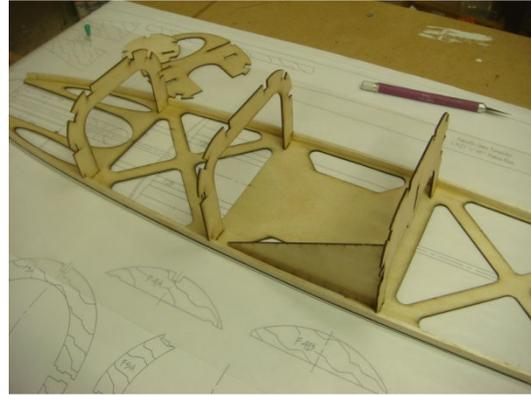
Glue F1 through F9 to the crutch, using the gauge to set them at the correct angle.
