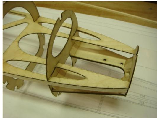
Glue the L.G. mount in place and reinforce it with triangle stock. Glue F1A, F1B, F2B, F4A, F4C, WS1, and WM1 in place.
