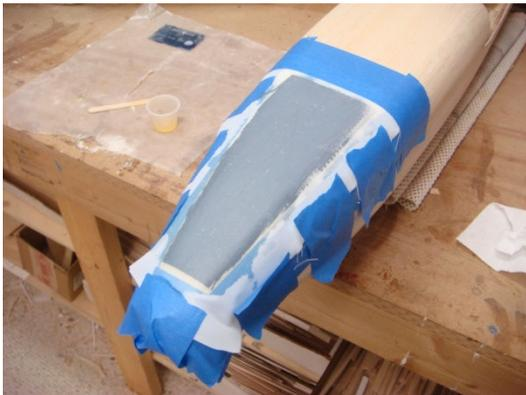
The front L.G. doors are laid up from fiberglass and carbon similar to the main gear doors.
