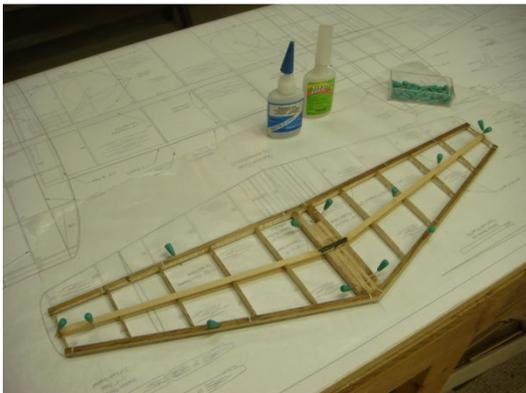
The stabilizer is built up over the plans. Position two basswood spars over the plans and glue the ribs in place. The spar will not be flat on the board. Glue the top spars, and the leading edges (L.E.) and trailing edges (T.E.) to the ribs. Sand the T.E. to match the ribs. Sheet the top of the stab with 1/32" balsa.
