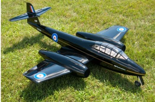
For landings, drop the gear on the downwind leg. The controls do get a little soft with the gear down, so just be aware of it. I make a long low approach and can cut power once on final. The Meteor does come in a bit hot, but it will stay down once it touches down. If you have to abort a landing attempt, retract the gear. It takes a considerable amount of power to get the Meteor back up to speed with the gear extended.
