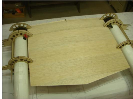
Sheet the bottom, center section of the wing with 1/16" balsa. Flip the wing assembly over, and support it in the jig blocks. Poke pins through the sheeting to mark the corners of the L.G. doors. Do not cut the door out at this time.
