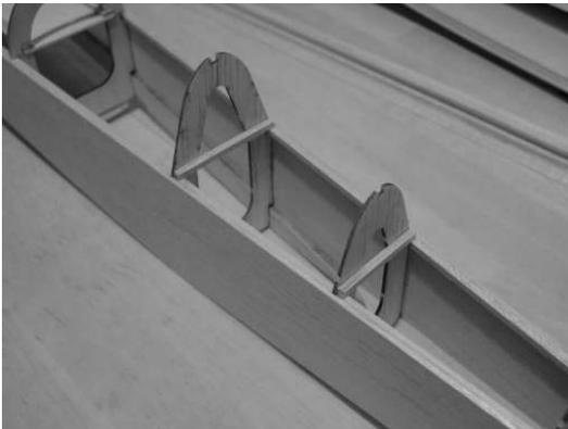
Glue in F6, F7, and F8. Cut and glue in place 1/8" square balsa cross braces for F6 and F7.
