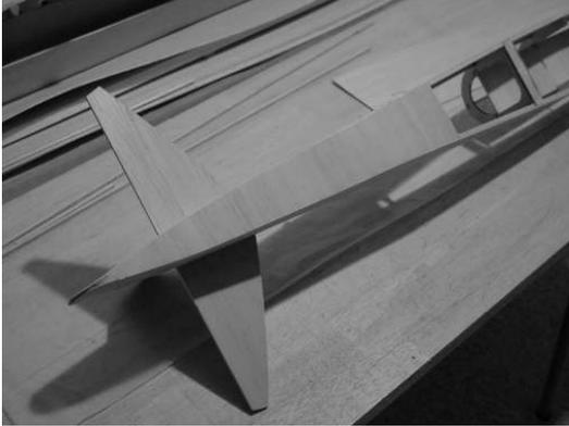
Cut 1/16" cross grain balsa for the lower rear sheeting and glue in place. Check the alignment of the fuselage with the plans as you go.
