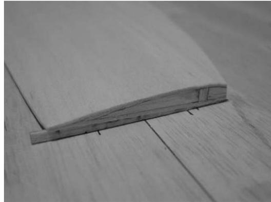
Using the washout jig under R10, re-pin the assembly to the board. Use a shim under the trailing edge at each rib location to create a gradual twist in the wing from R4 to the tip. The upper wing sheeting runs from R2 to R10. Cut and glue the upper wing sheeting in place.
