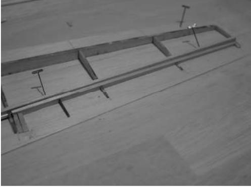
Frame in the aileron with 1/8" balsa for the L.E. and 1/4" balsa for each end. Notch the leading edge for the torque rod. Offset the end pieces 1/32" from R7 and R10. Use scrap balsa to reinforce the torque rod in the aileron but do not glue the torque rod to the aileron at this time. Glue in the aileron portions of R8 and R9. Mark the location of the aileron with pin holes in the lower wing sheeting.
