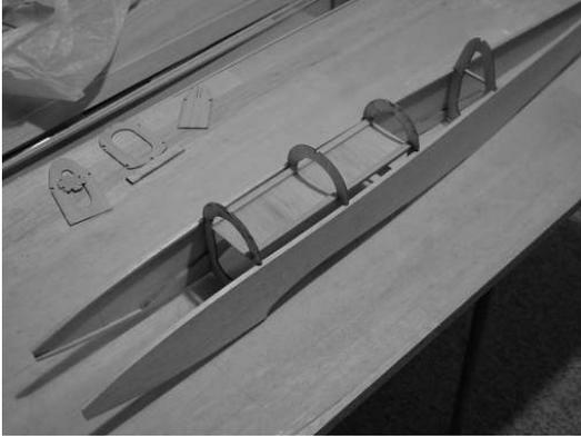
Glue F3, F4, and F5 to one side. Insert, but do not glue, the battery tray into F3, F4, and F5 being careful with F4. Glue the other side to F3, F4, and F5. The battery tray will help keep F4 from being crushed during this stage.
