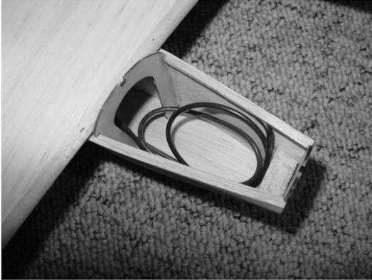
Fill in the lower front of the nacelle with balsa block. Glue the 1/2" balsa nacelle bottom in place and carve/sand the nacelle to shape. Repeat these steps to build the other nacelle.
