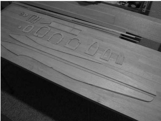
Cut out two fuselage sides from 1/16" balsa. Mark the locations of the formers. Glue the 1/8" square balsa stringers
