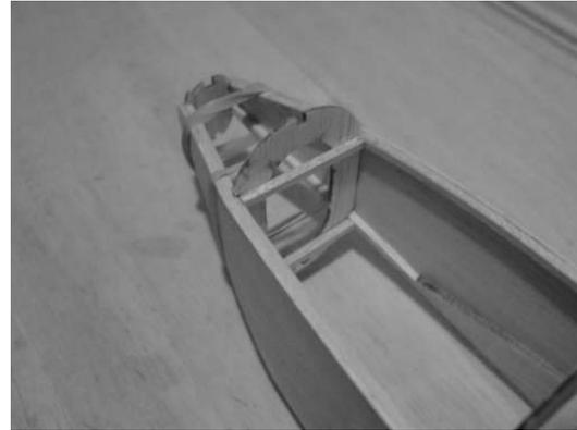
Cut and glue two 1/8" square balsa cross braces to F2. Glue F2 in place. You may need to wet the fuselage sides and use some rubber bands to hold the sides together. Glue F1 in place and use some more rubber bands to hold the fuselage sides together.
