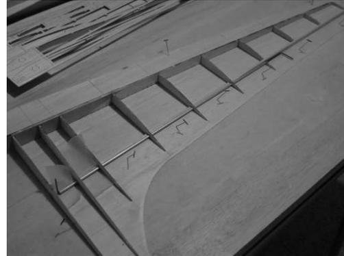
Thread the torque rod assembly into the holes in R7 to R2.
