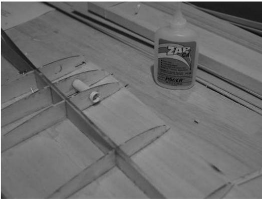
Keeping the rear portion of the sheeting flat on the board and the main spar square to the sheeting, glue the forward portion of R1 to R10 to the main spar ONLY. Use scrap balsa under the front lower sheeting to bend it up to meet the ribs. Use thin CA to glue the sheeting to the ribs. Install a paper tube between R2 and R3 for the motor wires.
