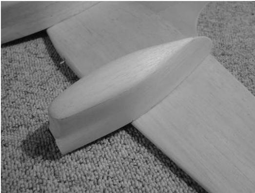
Make any necessary adjustments before permanently gluing the nacelles in place. Install the motors and connect the wires. When everything is set, glue in the 1/8" balsa N3 and plank the top of the nacelle with 1/16" balsa. Protect the wing with masking tape while you final
