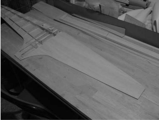
Remove the wing assembly from the board and build the other half onto it. One wing tip should be blocked up 2 1/2" to set the dihedral. Add scrap balsa reinforcement to each side of the R1's to make a pocket for the wing mount dowel. After the second half is sheeted, the center top wing sheeting can be cut to size and glued in place from one R2 to the other R2.
