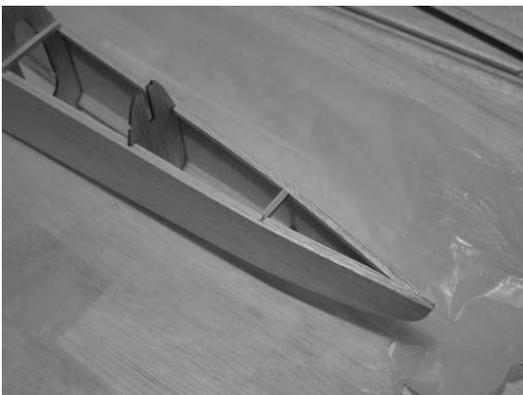
From the plans add the rear 1/8" square balsa cross braces at the tail. Sand the triangle stock to shape at the tail. Square up the tail and glue the two fuselage sides together.
