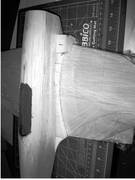
Figure 19 – Foam blocks added to fillet base
