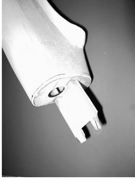
Figure 21 – Motor mount completed
