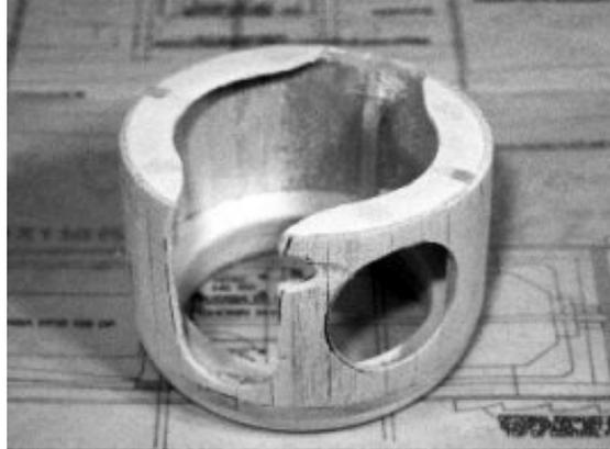
Cowl trimmed to clear engine and muffler, as well as allow air to exit either side. Earlier version shown here.
