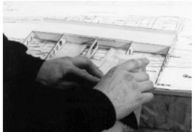
Sanding bevel on underside of **TE-MU**
