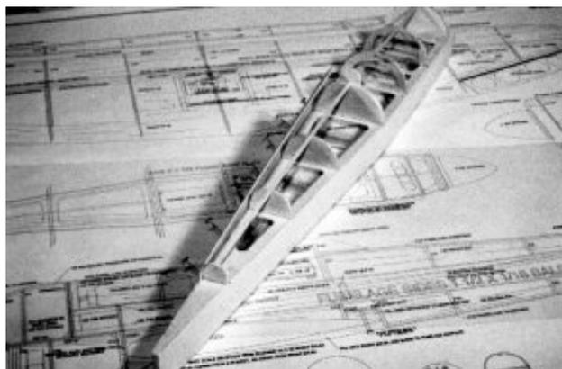
**URFS** glued along top edge of central fuselage box
