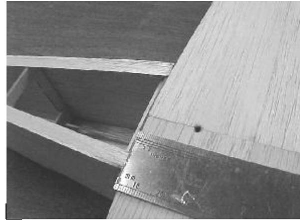
39. Measure forward from the trailing edge 1/4" and drill a 3/32" diameter hole thru the wing and ply plate. Bolt the wing in place with a #4-40 screw and blind nut.
