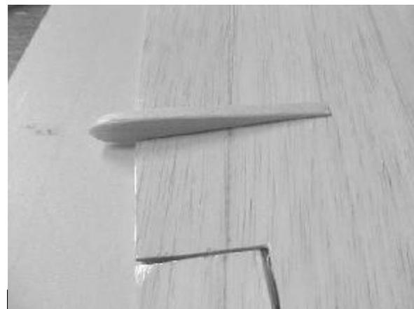
52. Make up the flap tracks using the pattern on the plan.
