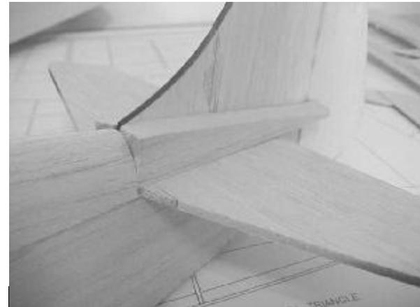
48. Use the tail surfaces as spacers and glue the balsa tail blocks to the fuselage only!
