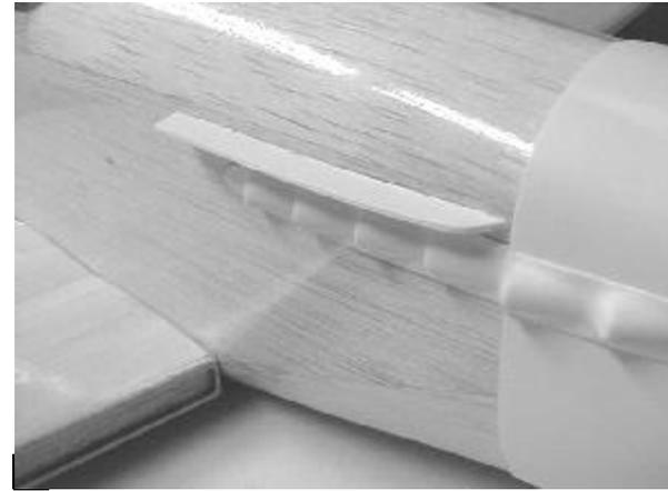
55. Cut the exhaust shields from scrap plastic and glue just above the exhaust stacks.
