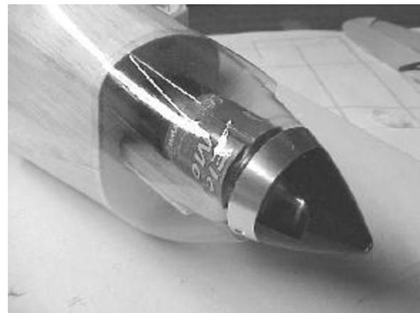
51. Rubber band the motor to the spruce rails, put the cowl and spinner in place and adjust the gap. With everything set glue the spruce rails from inside the wing opening.
