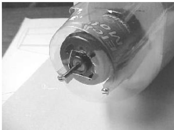
50. Cut 2 pieces of 1/4" x 1/4" spruce 4-1/4" long and slip them into F1, F2 but do not glue. Set the motor in place and fit the cowl, use the spinner to get it in place. When it is lined up mark the screw locations, drill holes and screw the cowl to the spruce rails with #2 screws. Note the 1/16 balsa on the underside of the rails.
