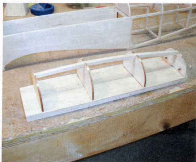
The basic top hatch cover is shown here ready to be planked with balsa strips.
